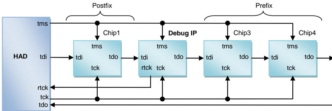
The example target shown in the figure above consists of the DoCD Debug IP and three, fully JTAG compliant devices. The Chip1 has 5-bit long IR (Instruction Register), Chip3 IR's has 3-bit long and Chip4 has 4-bit long IR. A DR (Data Register) is always 1-bit long, for each JTAG device.
